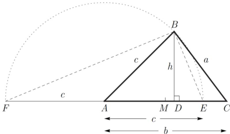
$$\begin{aligned} h^2 &= DE(2c - DE) = \left(c - \frac{b}{2} - \frac{c^2 - a^2}{2b}\right) \left(c + \frac{b}{2} + \frac{c^2 - a^2}{2b}\right) = \\ &= \frac{2bc - b^2 - c^2 + a^2}{2b} \cdot \frac{2bc + b^2 + c^2 - a^2}{2b} = \\ &= \frac{a^2 - (b - c)^2}{2b} \cdot \frac{(b + c)^2 - a^2}{2b} = \frac{(a + b - c)(a - b + c)(b + c + a)(b + c - a)}{4b^2} \\ S &= \frac{1}{2}bh = \frac{1}{4}\sqrt{(a + b - c)(a - b + c)(b + c + a)(b + c - a)} \end{aligned}$$
