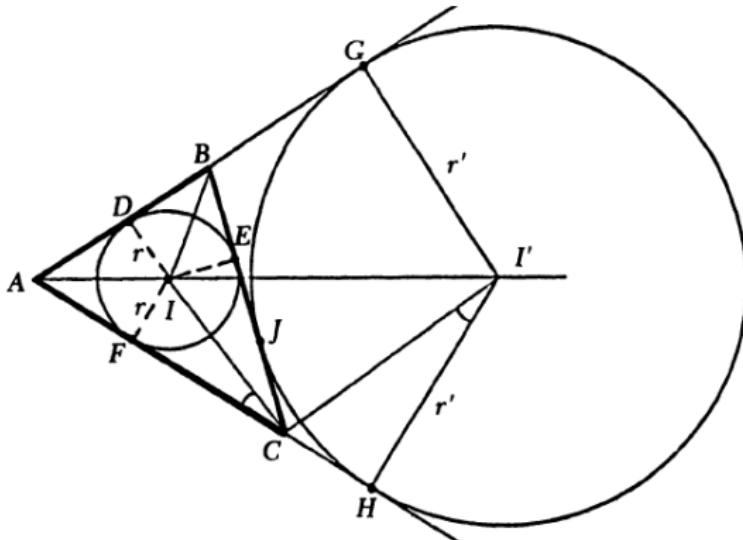
$$\begin{aligned} AG + AH &= (AD + DB + BG) + (AF + FC + CH) = \\ &= (AD + DB + BJ) + (AF + FC + CJ) = (AD + DB) + (BJ + CJ) + \\ &\quad +(AF + FC) = c + a + b = 2s \quad \Rightarrow \quad AG = AH = s \end{aligned}$$
